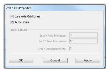
The option to display graph lines for each axis can also be selected in Axis Properties window.
