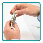
Remove the battery. If it is not sticking out for you to easily grab and pull, it may be stuck. Try giving it a shake and it should come loose.
