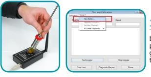
**11** Place the logger in the interface. In DTPro in the Test and Calibration window, click the "New Battery" button under the "Tools" menu. Follow the on-screen prompts to reset the battery and perform a "test logger." The new battery is now successfully installed and the logger is now ready for use.
