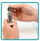
**3** Open up the housing. You'll notice that this lifts away. Try not to pull it too far back because there is a ribbon cable here that can become damaged. The board could also become loose if it gets pulled too hard.
