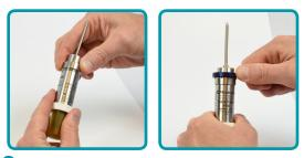
**10** Seal the logger. Use the lock ring and gripper tool to carefully slide it over the probe to get it into place. Hold it loosely and begin screwing the lock ring down first. Once the lock ring is done, you can put some compression on the upper and lower housing and use the gripper tool or Locking Ring Wrench to tighten it. Remove the gripper tool from the logger and you have successfully changed the MPRF battery.
