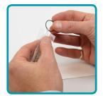
**7** Prepare the replacement O-Ring. Get a little bit of the grease from the o-ring removal tool kit and put some on your fingers. You will only need a small amount. We recommend rubbing the grease between your middle finger and thumb, and then slowly pulling the O-Ring through your fingers to allow the grease to completely cover it. It helps to have a paper towel nearby to wipe your hands once you are done.
