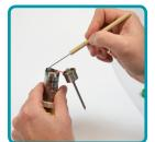
**5** Change the O-Ring seal. Use the O-Ring removal tool to poke into the O-Ring and remove it from the groove. You want to get the sharp end in as tightly as you can, then push down, and then push it to the side so it lifts up and out of the groove. Then use the tool to pull the O-Ring out completely. *Please note that any time you open the MPRF, you must replace the O-Ring with a new one.*
