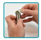
**9** Carefully slide the greased O-Ring over the housing. When it gets near the bottom, you will need to slightly stretch it to get it over the lip on the housing. Carefully push it into the groove. You should not need a lot of force, and rolling your finger around on the O-Ring will help if needed.
